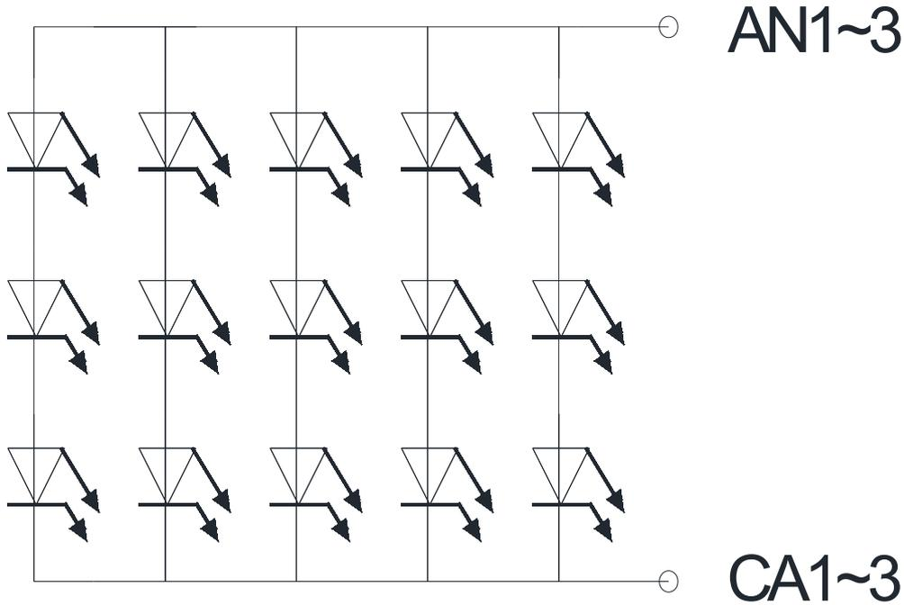
Note: AN1 to an3 are connected together inside backlight, CA1 to CA3 are connected together inside backlight. Forward current means the total current of the backlight, not the current of single string.
