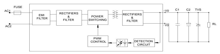
Note; The power supply is considered a component which will be installed into a final equipment. The final equipment must be re-confirmed that it still meet EMC directives.
